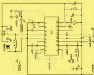
The antenna (Y) is a loose wire that should always be left unconnected and spread out for best radio reception.
