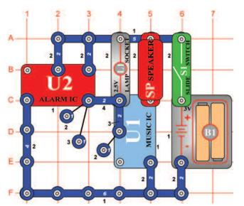
Build the circuit shown on the left and turn it on. The lamp (L1) alternates between being on and off while the speaker (SP) alternates between two musical tones... like someone is flipping a switch, but at a very consistent rate. Periodic signals like this are very important in electronics.
