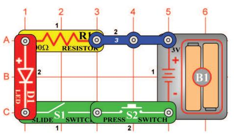
Build the circuit shown. Notice that if you turn on the slide switch (S1) AND press the press switch (S2) the LED (D1) lights up. Once again, there is no partially lit state here, the LED is either totally on or totally off. Two switches like this may be used to turn on the same light in your house, the room switch and the master switch in the electrical box. You could also have more than two switches and the circuit would function the same way.
