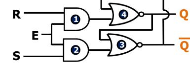
The Enable input (E) can be used as a clock input, or a read/write strobe.
