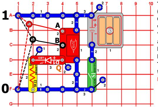
This circuit demonstrates how the NOR Gate (U19) works. Turn the slide switch (S1) on. Connect the loose ends of the red and black wires to either low voltage (denoted as a "0") or high voltage (denoted as a "1"). If, and only if, both input A AND input B are low (0), then the Q output on U19 will be high (1), and the red LED (D1) will be on. The output logic is exactly the opposite of the OR gate, hence this gate is called the NOT OR or NOR Gate.
