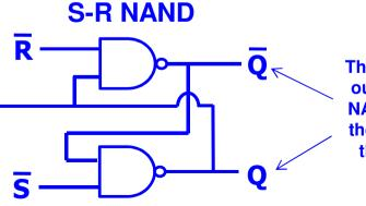
This shows that outputs of S-R NAND latch are the opposite of the S-R NOR latch
