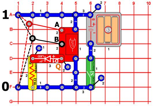
This circuit demonstrates how the OR Gate (U17) works. Turn the slide switch (S1) on. Connect the loose ends of the red and black wires to either low voltage (denoted as a "0") or high voltage (denoted as a "1"). If either input A OR input B are high (1), then the Q output will be high (1), and the red LED (D1) will be on.
