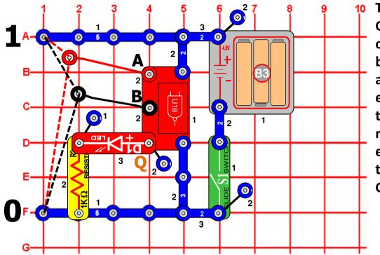
This circuit demonstrates how the NAND Gate (U18) works. Turn the slide switch (S1) on. Connect the loose ends of the red and black wires to either low voltage (denoted as a "0") or high voltage (denoted as a "1"). If either input A OR input B are low (0), then the Q output on U18 will be high (1), and the red LED (D1) will be on. The output logic is exactly the opposite of the AND gate, hence this gate is called the NOT AND or NAND Gate.
