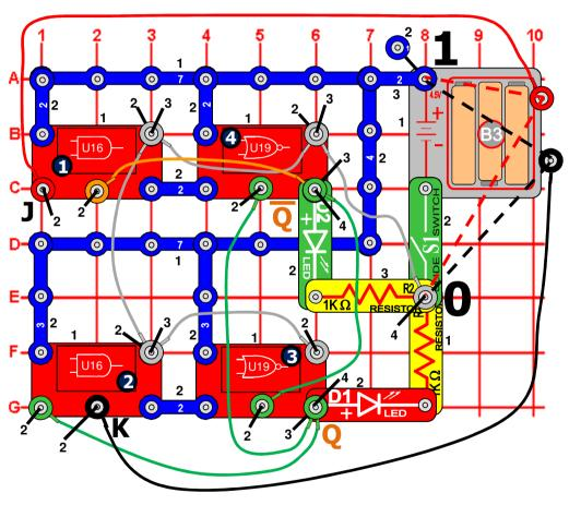
This circuit demonstrates how a J-K Latch works. Turn the slide switch (S1) on. Connect the loose ends of the red and black jumper wires to either 0 or 1.
