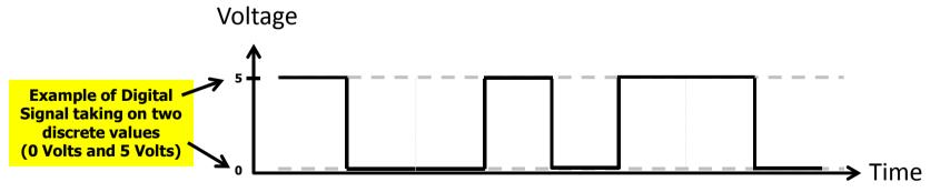
Analog signals can take on a continuum of values while digital signals take on only discrete values.
