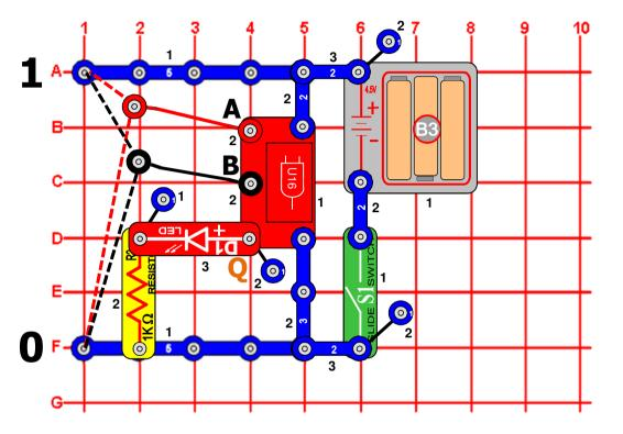
This circuit demonstrates how the AND Gate (U16) works. Turn the slide switch (S1) on. Connect the loose ends of the red and black wires to either low voltage (denoted as a "0") or high voltage (denoted as a "1"). If, and only if, both input A AND input B are high (both 1s), then the Q output will be high (1), and the red LED (D1) will be on.
