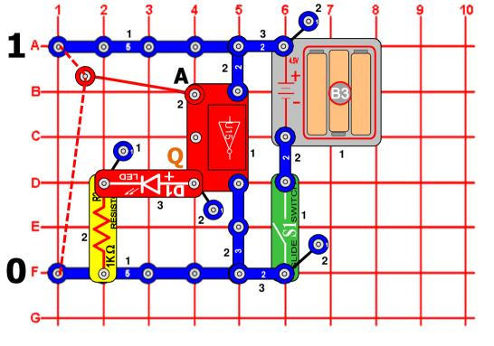
This circuit demonstrates how the NOT Gate (U15) works. Turn the slide switch (S1) on. Connect the loose end of the red wire to either low voltage (denoted as a "0") or high voltage (denoted as "1"). If input A is low (0), then the Q output will be high (1), and the red LED (D1) will be on. If input A is high (1), then the Q output will be low (0) and the red LED will be off.
