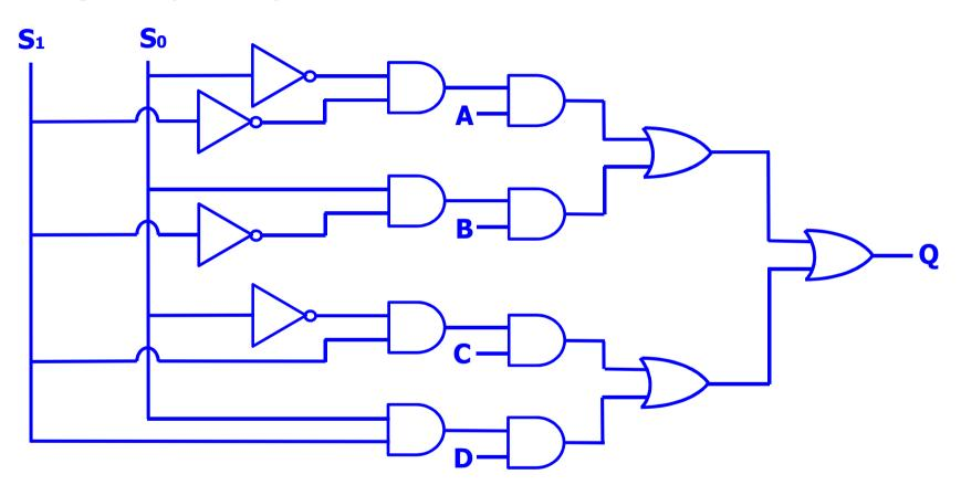
When  $S_0=S_1 = 0$ , then Q=AWhen  $S_0=1$ ,  $S_1=0$ , then Q=BWhen  $S_0=0$ ,  $S_1=1$ , then Q=CWhen  $S_0=S_1=1$ , then Q=D
