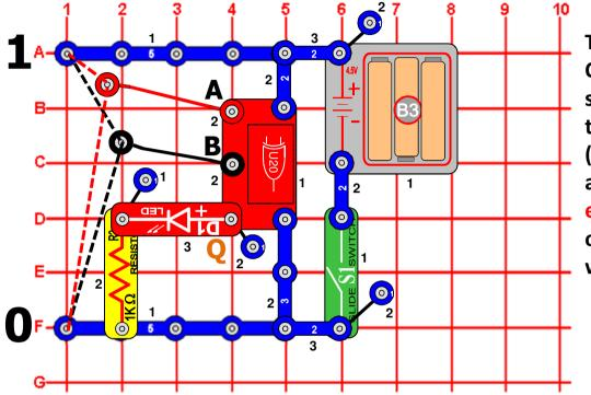
This circuit demonstrates how the Exclusive OR (XOR) Gate (U20) works. Turn the slide switch (S1) on. Connect the loose ends of the red and black wires to either low voltage (denoted as a "0") or high voltage (denoted as a "1"). If input A and input B are exclusive (i.e. different), then the Q output on U20 will be high (1), and the red LED (D1) will be on.
