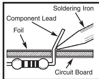
2. Apply a small amount of solder to the iron tip. This allows the heat to leave the iron and onto the foil. Immediately apply solder to the opposite side of the connection, away from the iron. Allow the heated component and the circuit foil to melt the solder.
