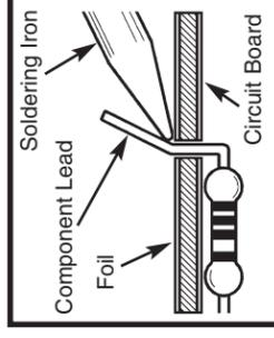
1. Solder all components from the copper foil side only. Push the soldering iron tip against both the lead and the circuit board foil.
