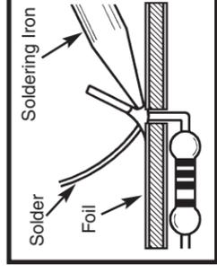
3. Allow the solder to flow around the connection. Then, remove the solder and the iron and let the connection cool. The solder should have flowed smoothly and not lump around the wire lead.
