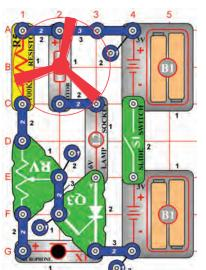
OBJECTIVE: To build a sound activated fan.
