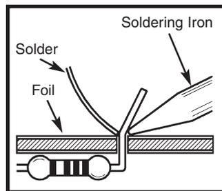
3. Allow the solder to flow around the connection. Then, remove the solder and the iron and let the connection cool. The solder should have flowed smoothly and not lump around the wire lead.
