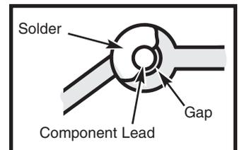
3. **Excessive solder** - could make connections that you did not intend to between adjacent foil areas or terminals.
