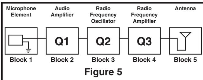
Block 2 is a transistor (Q1) used as an audio amplifier. The signal from the microphone element is increased in amplitude by a factor of 3. In electronics, this action is described as transistor Q1 having an audio gain of 3.
