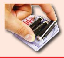
When installing a battery, be sure the spring is compressed straight back, and not bent up, down, or to one side.
