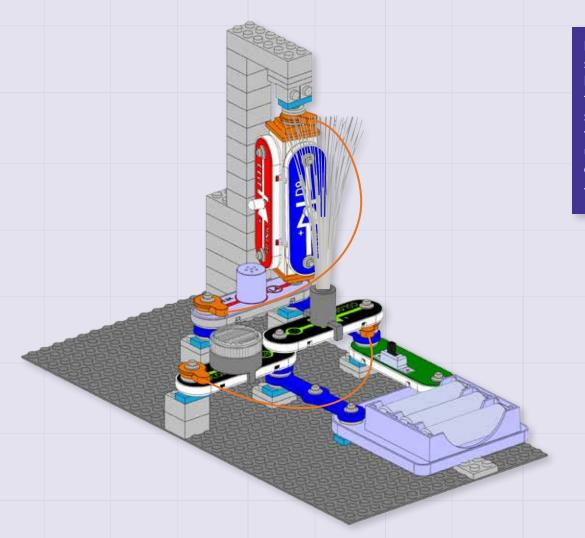
Build the circuit as shown, and turn on the slide switch (S1). The four LEDs (D8, D9, D11, & D12) and lamp (L4) light. The 3D snaps allow the blue and blink red LEDs to be rotated to shine in any direction. For best effects, place the fiber optic tree on the color2 LED (D12) using the mounting base, place the lined lens on the color LED (D8), and dim the room lights.
