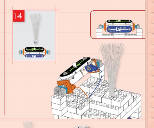
Build the circuit as shown, and turn on the slide switch (S1). The four LEDs (D8, D9, D11, & D12) and lamp (L4) light, and the melody IC (U32) plays tunes. The 3D snaps allow the blue and color2 LEDs to be rotated to shine in different directions. Dim the room lights for best effects.
