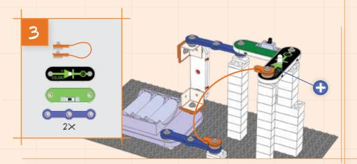
Build the circuit as shown, and turn on the slide switch (S1). The LEDs (D11 & D12) light in a blinking pattern. You can replace the LEDs with any other LEDs and see how the circuit changes.
