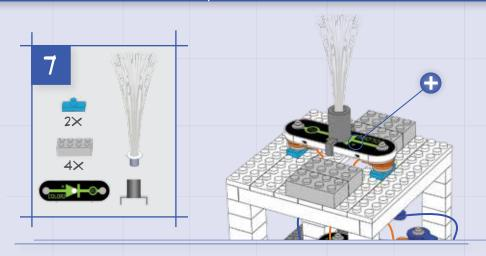
Build the circuit as shown, and turn on the slide switch (S1). The four LEDs (D8, D9, D11, & D12) and lamp (L4) light. Dim the room lights for best effects.
