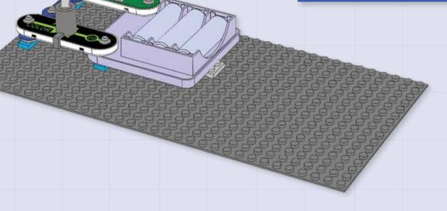
Snappy says when you turn on the slide switch, electricity flows from the batteries, through the color LED and back to the battery through the switch. If the switch is off, the flow of electricity is blocked, and the color LED won't light.
