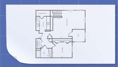
An architect's drawings may show the floor plan or other information about the construction, depending on who will be using the drawing. These drawings used to be call blueprints, due to the color used when making them years ago. Notice that the symbol for a switch in electrical schematics is based on the architect's symbol for a door.
