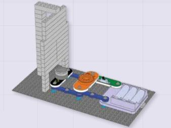
Build the circuit as shown, and turn on the slide switch (S1). The color LED (D8) shines a colorful pattern on the wall of bricks, for best effects rotate the lined lens so its lines converge toward the wall, and place the circuit in a dark room.
