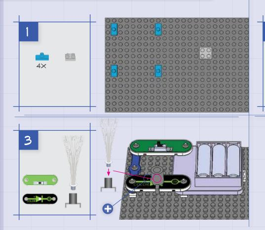
NOTE: this circuit (and many others in this book) have an LED being used without a resistor or other component to limit the electric current through it. Normally this could damage an LED but your Snap Circuits® LEDs include internal protection resistors, & will not be damaged. Be careful if you later use other electrical sets with unprotected LEDs. The festive tree and egg may also be used with other Snap Circuits® LEDs from different sets.
