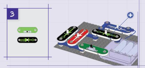
This circuit has two pairs of parallel LEDs in series with each other. Some of the LEDs are blinking in different patterns (D11 turning on and off, D8 changing colors quickly, and D12 changing colors slowly). Red color is easier to produce than green or blue, and green is easier to produce than blue. The combination of these effects creates the pattern you see.
