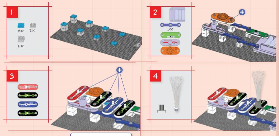
This circuit has the melody IC (U32), blink red LED (D11), and lamp (L4) connected in series, to show the differences in how they operate.
