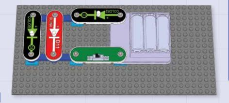
Here the color LED and blink red LED are connected in parallel, and then connected in series with the color2 LED, to produce some interesting effects. The electricity from the batteries flows through the color2 LED, then splits up between the color and blink red LEDs, then recombines in the switch before returning to the batteries.
